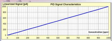
PID signal after linearization
